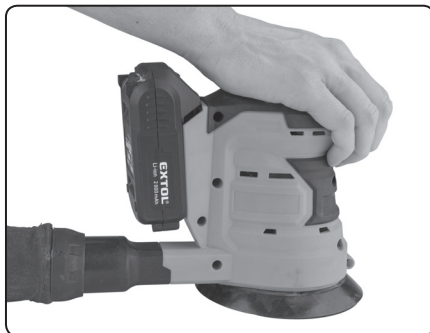
Fig. 5, guiding the sander over the sanded surfaces by hand
