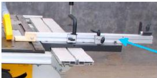
Cross cutting fence
